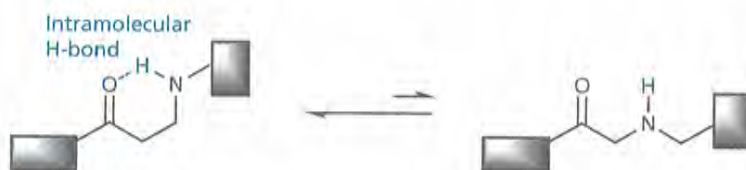
FIGURE 13.59 Rigidification involving an intramolecular hydrogen bond.
