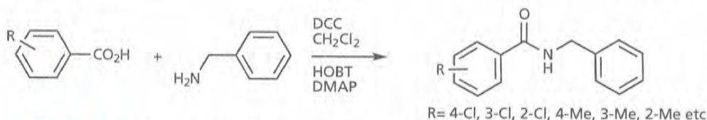
FIGURE 16.25 Coupling reaction of a carboxylic acid and an amine to give an amide library (DCC = dicyclohexylcarbodiimide, DMAP = dimethylaminopyridine, HOBT = hydroxybenztriazole).
